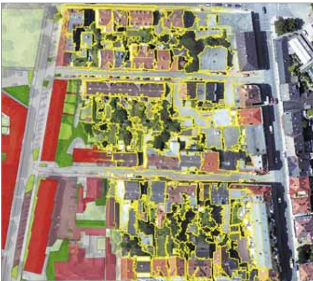
Automated remote sensing: similar pixels in one aerial photograph (right) are automatically combined into segments (centre), from which a data set of use types (left) can be compiled by classification
